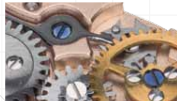
Maltese cross mechanism for a regular force transmission
