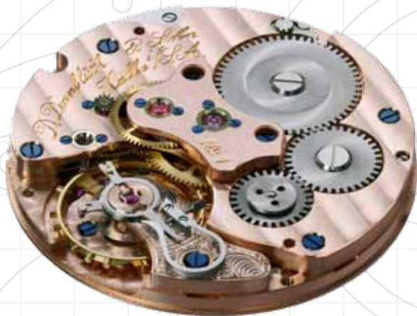
Ratchet wheels with a sunburst finish, flat polished ratchet and ratchet spring
