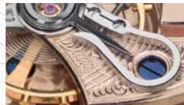
Fine adjustment with a swan-neck spring on a hand-engraved balance cock
